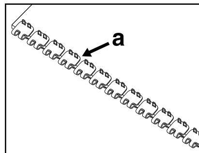
**3.** Place belt on solid surface for support. Center fastener strip, equal distance from the belt ends. (a) Staples should be facing up.
