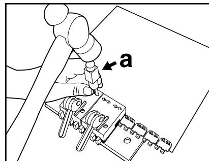
**6.** Starting with the center fastener plates, strike (a) staple driver with a 1 lb. (0.5 kg) hammer. Do not overdrive staples.
