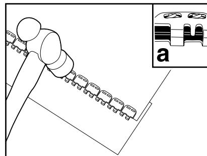
9. Set fastener strip flat on ST-28 setting plate. Strike top-side of fasteners and staples with firm hammer blows. Move back and forth across fastener strip until (a) staples clinch. Avoid hitting fastener loops. Repeat steps 1-9 on other belt end.
