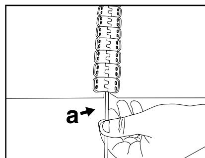
11. Bring belt ends together and (a) insert hinge pin. If retaining washer is used, crimp with pliers. Splice is complete.
